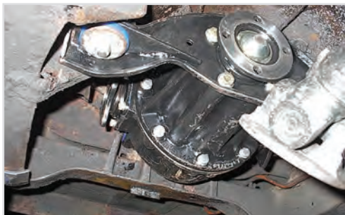
Newly Replaced Diff on my GT6, lots of scraped paint fitting it on my own!
