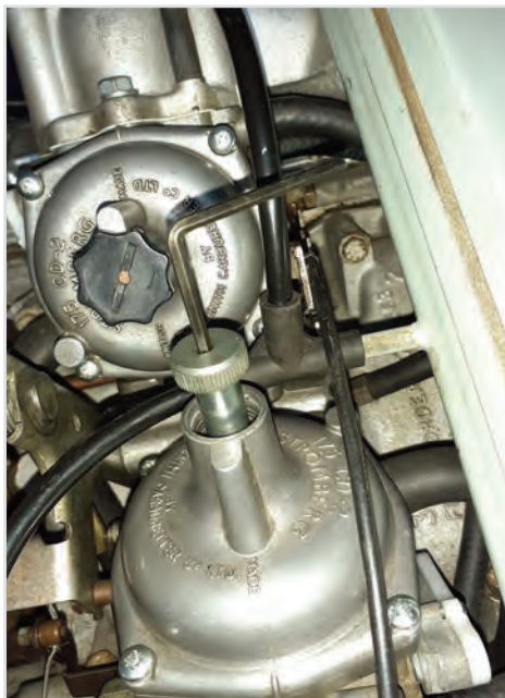
Pic 2. Adjusting the carb needle
