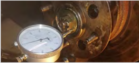
Checking the front wheel bearing end float with a dial gauge on my GT6
